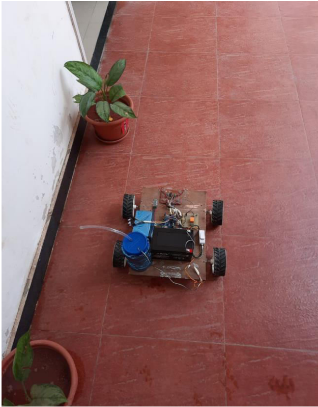
Fig.1. water pump start supplying water after sensing tag
